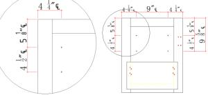
Step7: Must Predrill the Pilot Hole (1/4" Depth or less) on Face Frame of TB18. (Recommend 1/8" drill bit)
