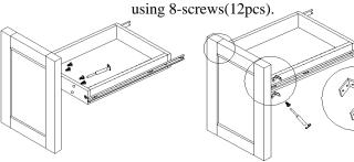
Step8-1: Mount long parts of (E) on Face Frame and Step8-2: Mount Rear Brackets of (E) on Back Panel, using 7-screws(4pcs).
